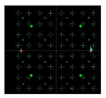
Figure 2: Constellation diagram of a downlink subframe with 4 different bursts with different modulation: BPSK (red), QPSK (green), 16QAM (blue) and 64QAM (yellow)
