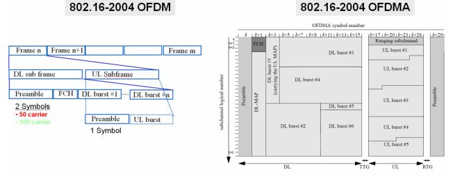
Figure 1: Comparison of frame structure of 802.16-2004 OFDM system and 802.16-2004 OFDMA. In OFDM e.g. the downlink consists of a preamble followed by an FCH field and the bursts for the different subscribers. In OFDMA mode the bursts are allocated according to downlink map.
